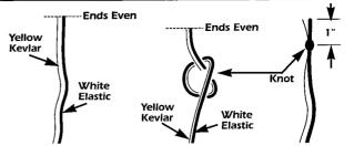
NOTE: THIS IS A VERY IMPORTANT STEP. IF YOU TIE A DIFFERENT TYPE OF KNOT THE SHOCK CORDS MAY SEPARATE DURING FLIGHT.
